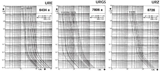
\* These curves indicate, for each rated current, the pearcing time vs. the R.M.S. pre-arcing current. \* Tolerance for the mean pre-arcing current  $\pm$  10%
