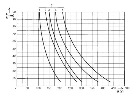
• These curve indicate the permissible value of time constant L/R as a function of the D.C. working voltage.
